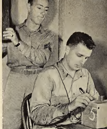
In steadiness test, Cadet Lionel Humphries holds a pin-sized stylus in a nail-sized hole as the instructor attempts to rattle him. If the stylus touches the hole, it records a demerit.
